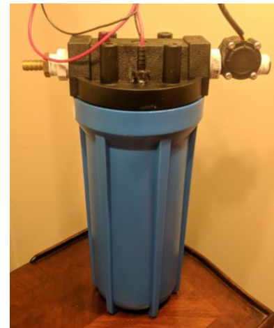
Figure 2: Electrochemical Chlorine Generation.
