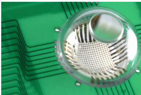
Figure 2. Electronic 'eyeball camera', consisting of a hemispherical photodetector array integrated with a simple imaging lens.
